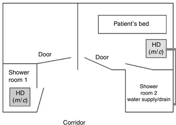
**Figure 1 | Schematic plan of section of oncology ward.** The dialysis machine was prepared in the adjacent shower room—shower room 1 using a potable water supply. The dialysis machine and portable reverse osmosis unit were then moved into the patient's room and connected to a potable water supply and drain from shower room 2.
